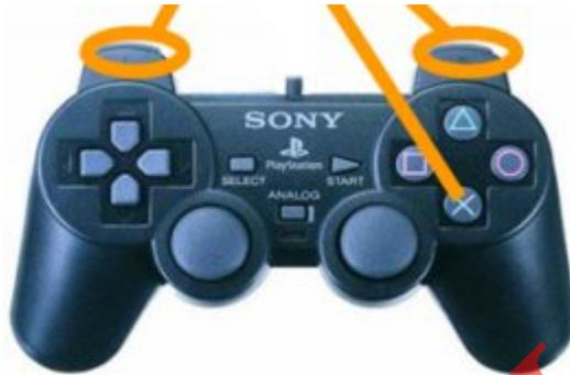
To enter this mode hold the **X, L1, L2, R1, R2** together for 5 sec while **WELCOME** is displayed on screen, then you will see words "**Engineer mode**".
